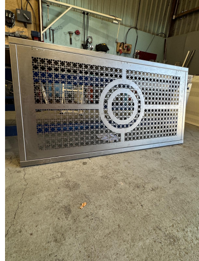
The 2mm steel panel in the workshop before finishing.
